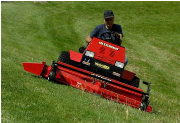
The compact, nimble Steiner 235 Tractor offers a low center of gravity for stability on undulating terrain and a tight 14-inch turning radius.
